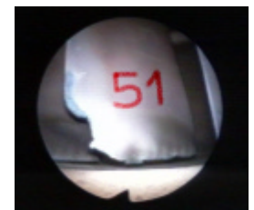
Figure 9 Vibration cause HPT blade deterioration
